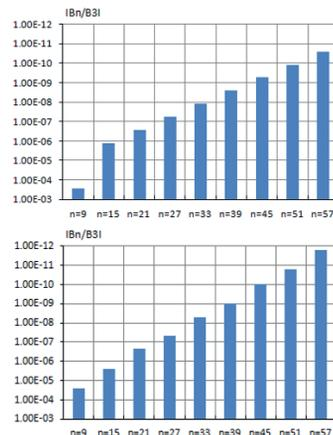
Figure 13: Normalized multipole errors of the sextupoles with 28 mm (up) and 23 mm (down) radius at +12 mm.
