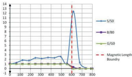
Figure 5: Relative deviation of fields on the central line along half of the dipole magnet.
