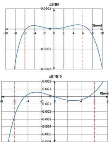
Figure 3: Field quality of the 2D designed dipole sections within ±6 mm GFR for both dipolar (up) and quadrupolar components (down).
