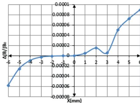
Figure 6: Integrated field quality of the SR dipole magnet in the  $y=0$  plane with chamfer.
