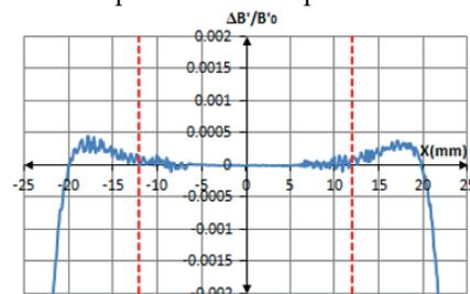
Figure 8: The field quality of the SR quadrupole within horizontal distance. The red dotted lines are GFR limits.
