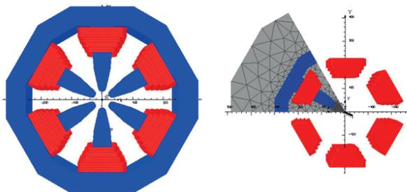
Figure 11: 3D design of the one of the SR sextupole magnets in OPERA with 28 mm aperture radius.
