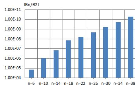
Figure 9: Normalized multipole errors at +12 mm.
