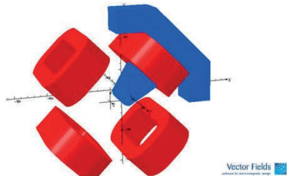
Figure 7: 3D design of the SR quadrupole magnets in OPERA.
