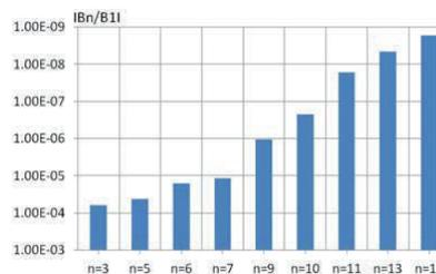
Figure 4: Normalized multipole errors of SR dipole magnet at +6 mm.
