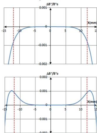
Figure 12: The field quality of the sextupoles with 28 mm (up) and 23 mm (down) aperture radius.
