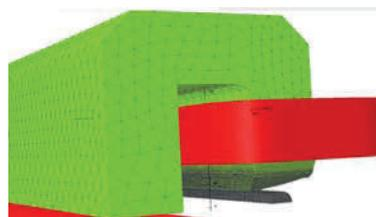
Figure 2: 3D design of the SR dipole magnets in OPERA.
