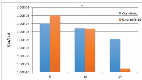
Figure 9: Absolute normalized integrated multipoles' errors at 12.5 mm GFR with (blue) and without (orange) chamfer.
