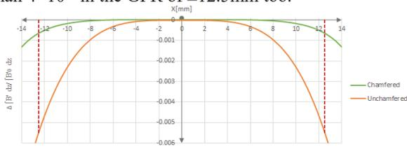
Figure 8: Integrated field quality of the booster quadrupole magnet in the  $y=0$  plane with and without chamfer.
