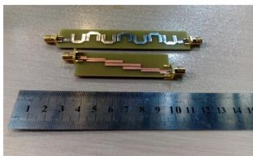
Figure 8: Fabricated filters on 1.6 mm FR4 substrate.
