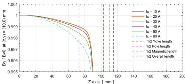
Figure 6: Prototype longitudinal field distributions.
