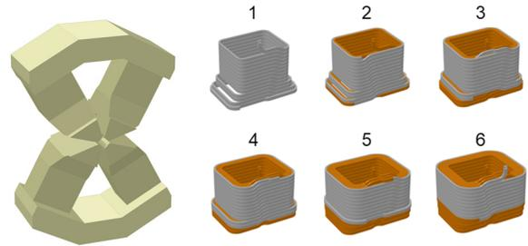
Figure 2: Quadrupole yoke and coil winding.
