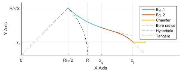
Figure 3: Pole profile equation and plot.
