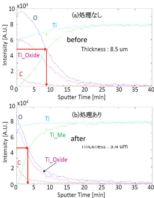
Figure 2: Measurements of the oxide film thickness before and after nitric hydrofluoric acid treatment measured by AES.
