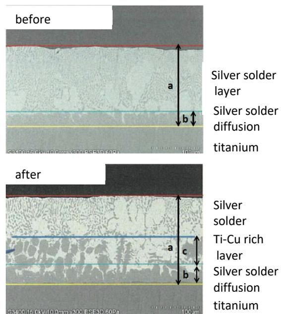
Figure 4: Cross section pictures of silver solder and pure titanium before and after heat treatment.
