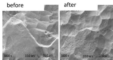
Figure 1: SEM Pictures of surface of the pure titanium before and after nitric hydrofluoric acid treatment.
