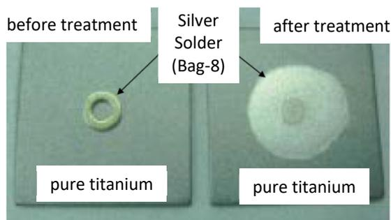
Figure 3: Pictures of the silver solder on the pure titanium surface before and after heat treatment. Outer diameter: 4.35φmm(before), ~11φmm(after), Inner diameter: 2.5φmm(before), 0mm(after).
