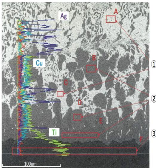
Figure 5: Elemental analysis of silver braze on pure titanium which was treated by nitric hydrofluoric acid after heat treatment measured by EDX.
