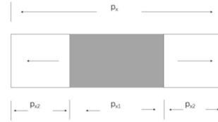
Figure 4: The transverse structure of the pole. The middle part is still CoFeV, and the ends are changed to magnets with different magnetization directions.
