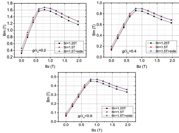
Figure 3: The peak magnetic field of SAU at different gaps. The curves with square remarks respect the peak field of SAU without side magnets and the  $B_r$  is only 1.25 T. The curves with circle remarks respect to that of the SAU with the  $B_r=1.5$  T but no side magnets. The curves with triangle remarks respect the SAU with side magnets and  $B_r=1.5$  T.
