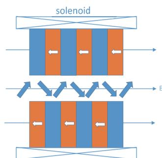
Figure 1: The structure of SAU. The magnetization direction of the magnet is opposite to the magnetic field of the solenoid.
