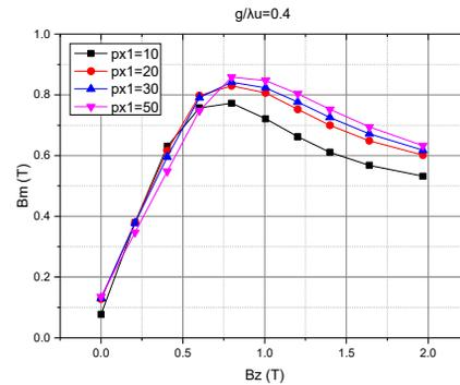
Figure 5: Peak magnetic field at different  $p_{x1}$ .
