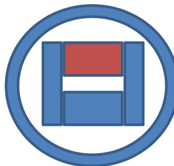
Figure 2: The structure of the cross section of SAU. The horizontal rectangles represent the magnetic pole and magnet of the SAU. The vertical rectangles represent the side magnets outside the SAU, whose magnetization direction is opposite to the solenoid. The outer ring represents the solenoid.
