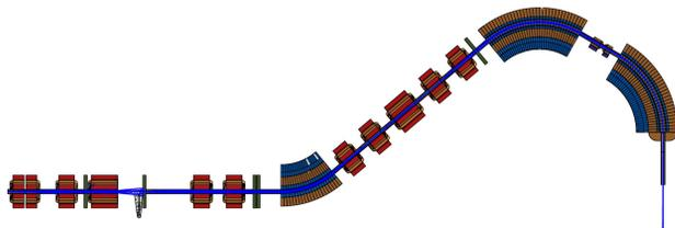
Figure 2: Complete model of the Proteus<sup>®</sup>One beam transport line made with BDSIM. The propagation of the proton beam is shown in blue. The secondary particles are not shown.
