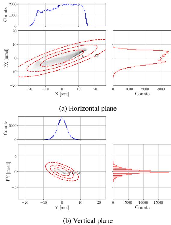
Figure 1: Phase space of the beam in both planes. The projection over each axis is also shown.
