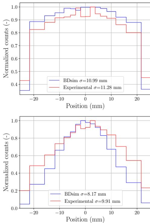
Figure 5: Comparison with experimental results at two positions in the beamline. The red line correspond to the experimental data and the blue line to the results obtained with our model.
