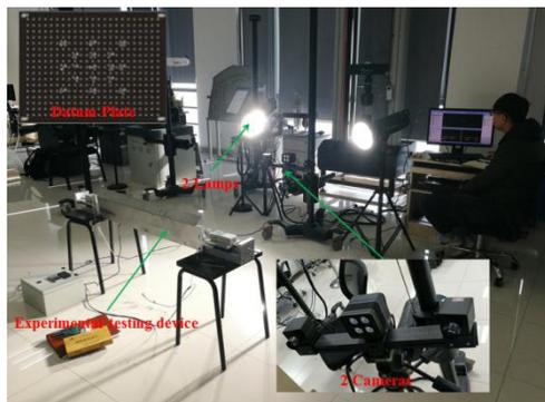
Figure 6 : 3-D imaging measurement system.
