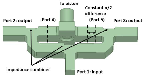
Figure 5: Geometry of RF power splitter (HFSS model).
