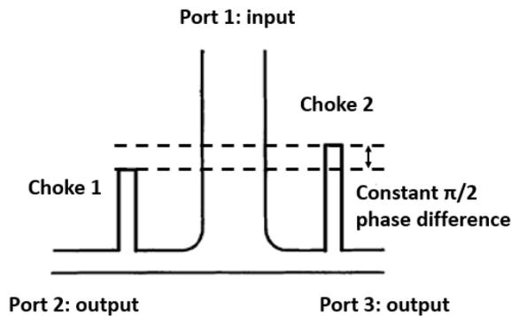
Figure 3: Schematic of RF power splitter.
