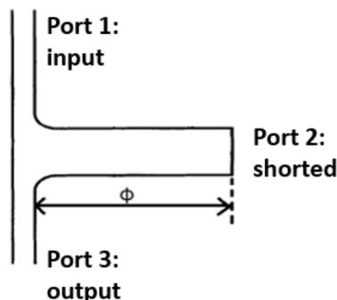
Figure 2: Schematic of choke-mode.
