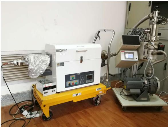
Figure 2: Experimental sintering device.
