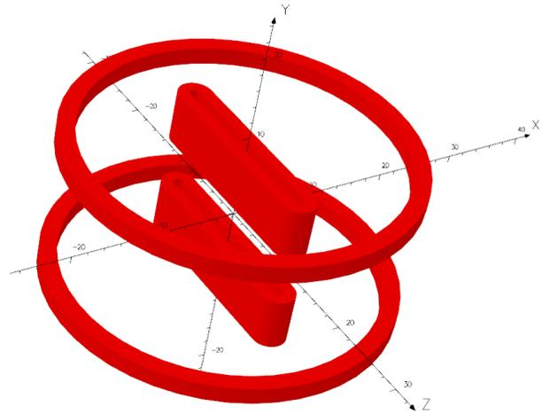
Figure 1: The structure of coils, beam travels along the Z-axis.
