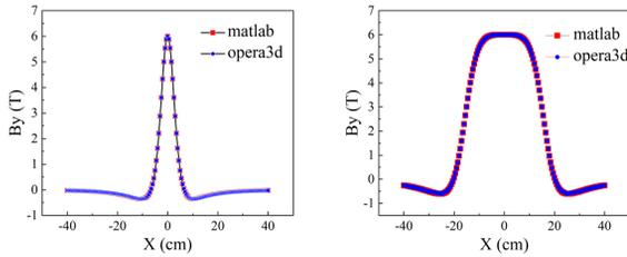
Figure 2: The parameters of inner coils are  $r_{in}=1$ ,  $w_{in}=2$ ,  $h_{in}=3$ ,  $t_{in}=6$ ,  $l_{in}=10$  and  $R_{out}=15$ ,  $W_{out}=2$ ,  $H_{out}=7$ ,  $T_{out}=2$  for outer coils. The scale is centimeter.
