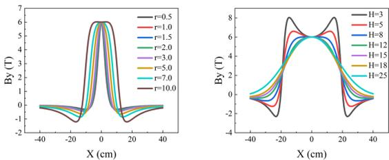
Figure 3: Vertical B-field along the beam path of inner coils (left) and outer coils (right).
