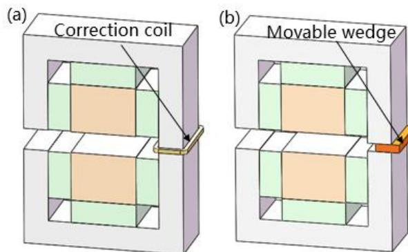
Figure 6: (a) Correction coil (b) Movable wedge used to tune field.
