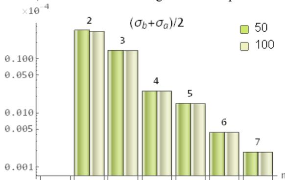
Figure 8: Stand deviation of the multipoles induced by magnetization direction error of 50 and 100 mrad.
