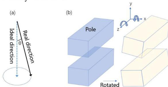
Figure 7: (a) Magnetization direction error of PM block; (b) Parallelism error due to rotation of poles.
