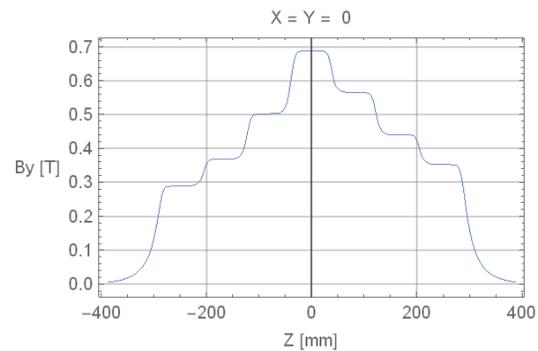
Figure 1: The fields of LGB versus longitudinal position.
