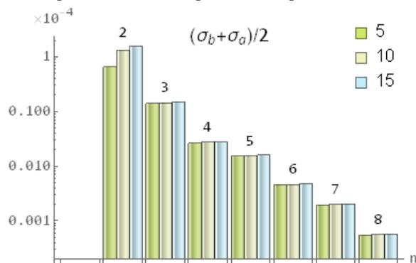
Figure 9: Stand deviation of the multipoles induced by parallelism error of poles of 5, 10 and 15 mrad.
