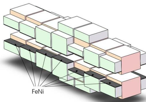
Figure 5: FeNi strips attached on the PM magnets.
