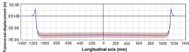
Figure 5: Transversal electrons excursion at 5.2 mm gap.
