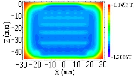
Figure 6: Demagnetizing field on the XZ surface of the magnet. Fields are always lower than 1.2 T.
