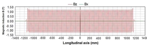
Figure 3: Magnetic field at 5.2 mm magnetic gap.
