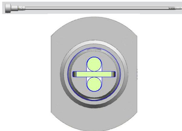
Figure 5: Lateral view (top) and cross-section (bottom) of the shaft.
