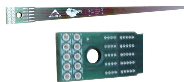
Figure 2: Multilayered PCB with the 5 coils.
