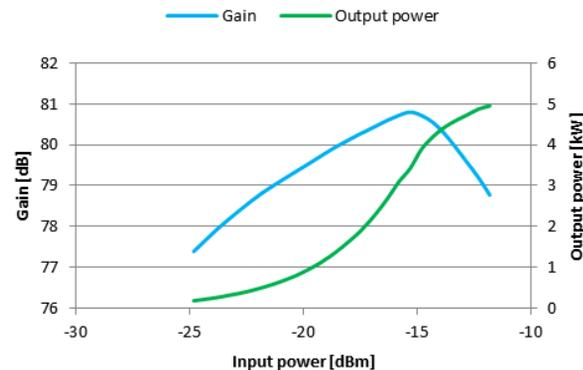
Figure 4: SSPA transmitter output power and gain.
