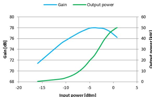
Figure 3: SSPA transmitter output power and gain.
