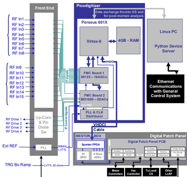
Figure 1: Main hardware components of Sirius DLLRF.
