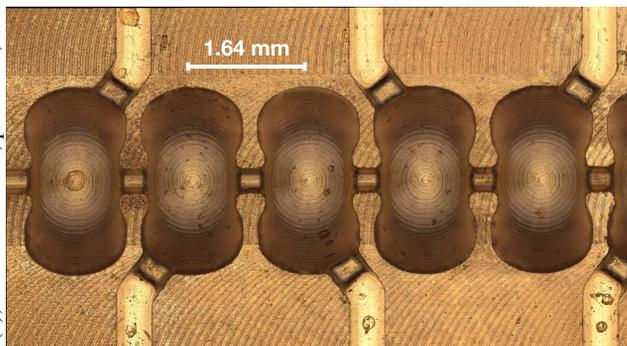
(a) 3D Microscope image of the five end cavities.
