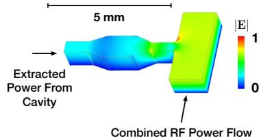
Figure 3: Electric field profile of the redesigned T-junction of the manifolds combining 20 cavities each.
