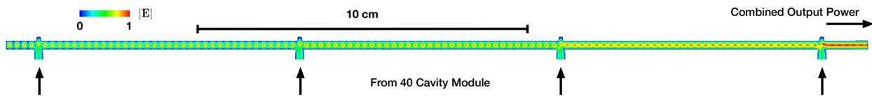
Figure 2: Electric field profile of the top-level manifold combining 4 sets of 40 cavities.
