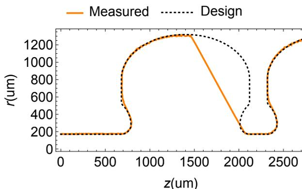
(b) Comparison of the measured nose cone profile with a 3D microscope and the design. Note that the 3D microscope can only measure depth and the structure was imaged tilted, hence only one side of the cavities could be imaged.
