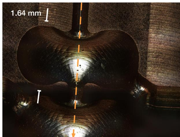
(a) 3D Microscope image of the two end cavities.
