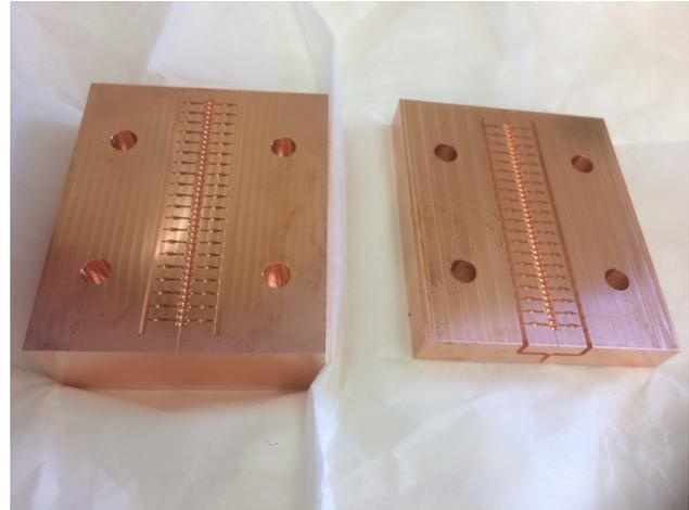
Figure 5: Picture of the bottom and middle block forming 40 cavities. Also shown is the splitter combining the two manifolds in the middle block.
