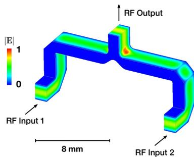
Figure 4: Electric field profile of the 3 dB combiner attached to the two bottom level manifolds, thus power-combining 40 cavities.
