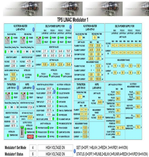
Figure 4: Graphic User Interface (GUI) for Linac Modulator.
