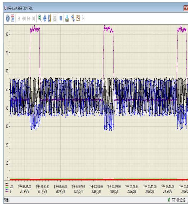
Figure 5: Historical data for RF pre-amplifier outputs at 4-minute top-up injection.
