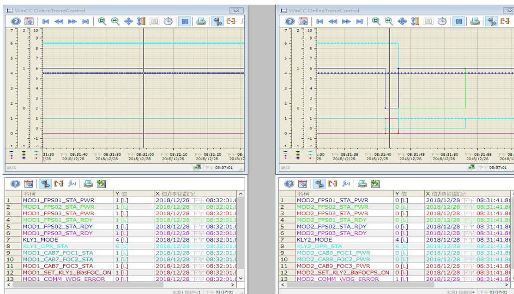
Figure 6: Archiving curves for all focusing magnet power supplies at normal operation (left) and system failure (right).
