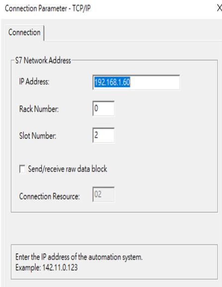
Figure 2: TCP/IP setting page in WinCC.
