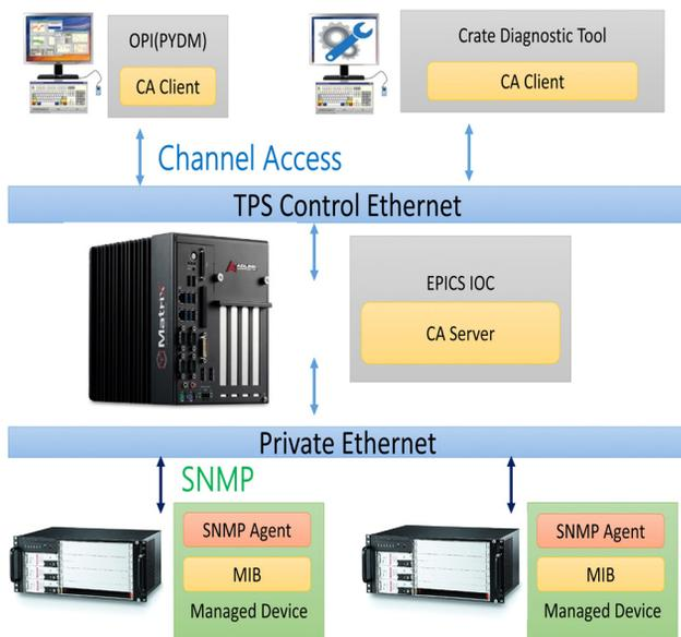
Figure 2: System structure of EPICS integrating an SNMP with a cPCI crate.
