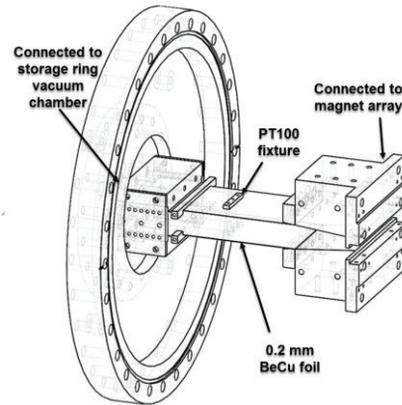
Figure 7: Transition taper for a CU15.
