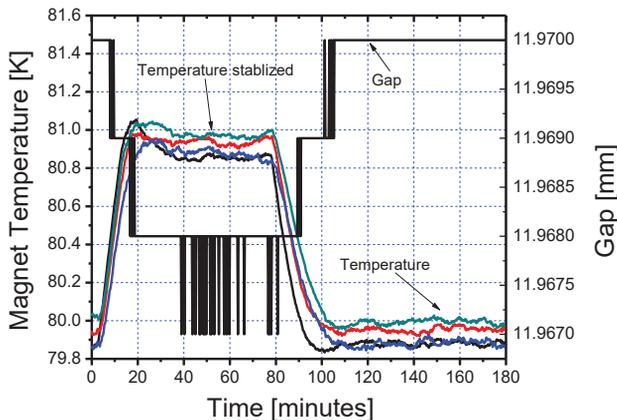
Figure 6: Time variation of undulator gap and temperature of the magnet arrays after the preset temperature change by 1 K.
