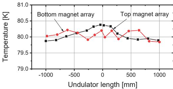
Figure 5: Temperature distribution along a magnet array with active temperature control system.
