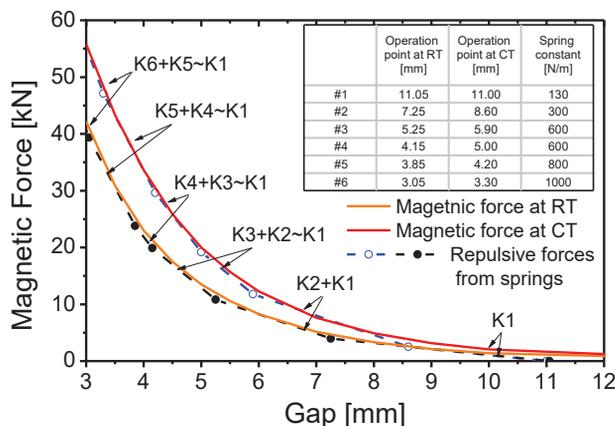
Figure 3: Dependence of magnetic (solid lines) and repulsive (dashed lines) forces as a function of gap size at 295 K and 77K.
