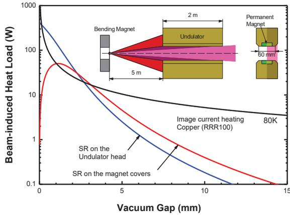
Figure 4: The beam-induced heat load (SR and IMG) The calculation is based on TPS parameters,  $E_{GeV} = 3$  GeV,  $I_b = 500$  mA, 600 bunches, bunch length = 4.65 mm (15.5 psec), circumference = 518 m, bending radius = 8.353 m and a distance of 5 m from the next upstream dipole magnet end to the undulator entrance.
