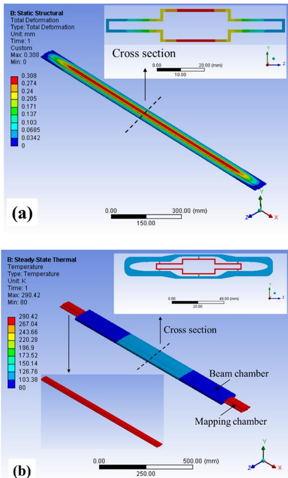
Figure 2: Mechanical strain and thermal simulation. (a) Deformation of mapping chamber under 1 atm pressure difference. (b) Temperature distribution of the SMPW after cool-down.
