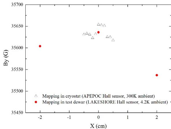
Figure 4: Field distribution along transverse direction mapping by the HPS in the cryogenic temperature and ambient room temperature.
