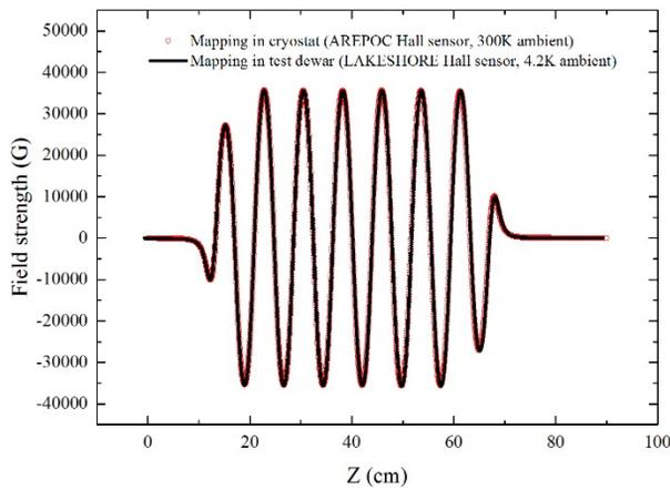
Figure 3: Field distribution measured with HPS along the magnet axis at room temperature and cryogenic temperatures.
