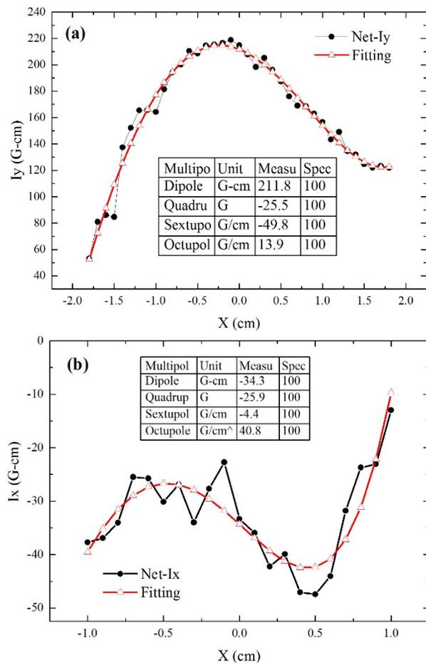
Figure 5: Field integrals measured with a stretched wire and fitted with a polynomial at room temperature in the cryostat. (a) Vertical field integral along the x-axis and (b) horizontal field integral along the x-axis.
