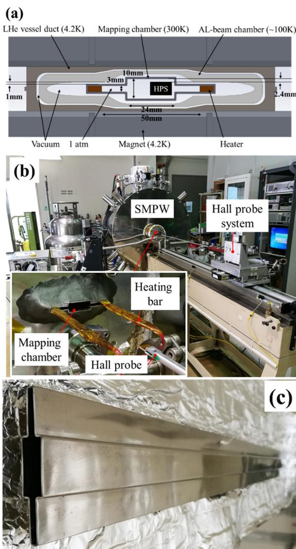
Figure 1: Field mapping at room temperature in a cryostat. (a) Sketch of the room temperature mapping chamber and cryostat. (b) Setup of the mapping system for the SMPW and (c) photo of the mapping chamber.
