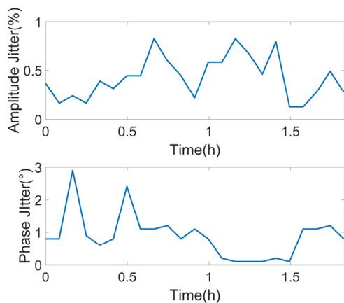
Figure 7: The amplitude and phase jitter of RF power.
