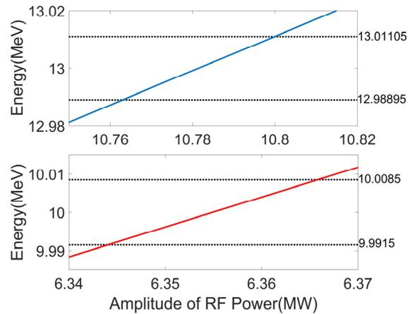
Figure 5: Electron energy increases with the increasing amplitude of RF power for selected beam energies.
