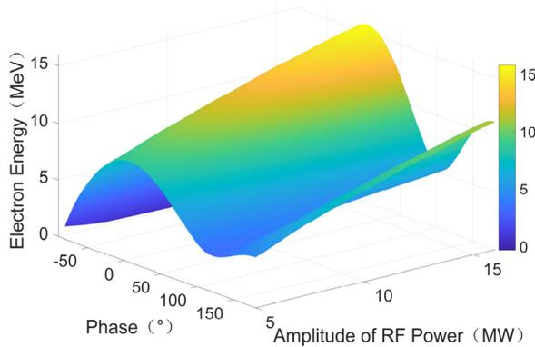
Figure 2: Fluctuation of electron energy with the increasing amplitude and phase of RF power.
