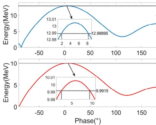
Figure 3: Electron energy fluctuates with the increasing phase and the RF power for selected beam energies.
