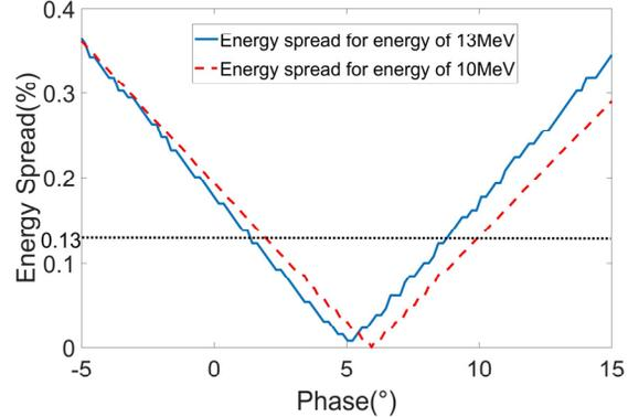
Figure 4: Energy spread change with the increasing phase.
