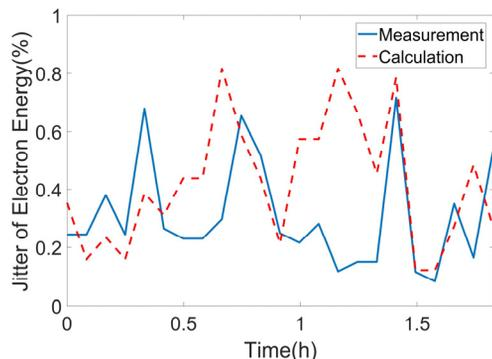
Figure 8: Calculated and measured jitter of electron energy.
