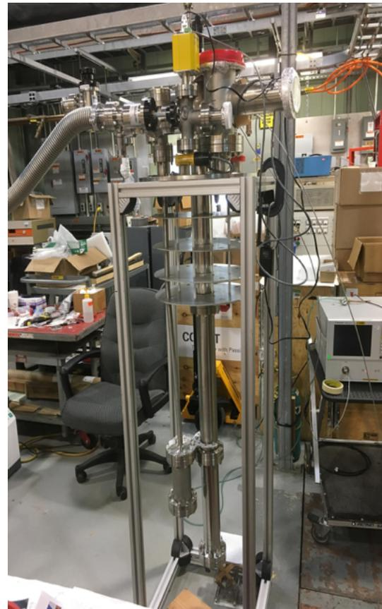
Figure 2 The BNL assembled cryogenic resonator.
