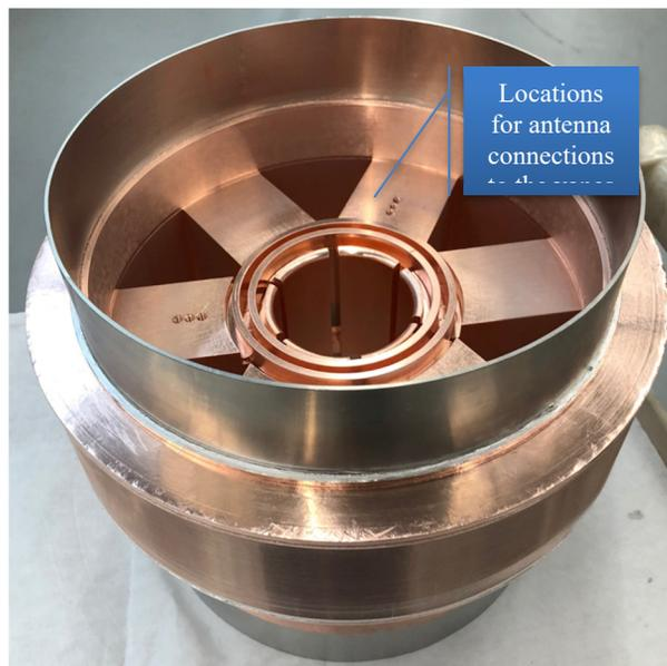
Figure 2: 350 MHz magnetron Anode ready for Qext measurements.
