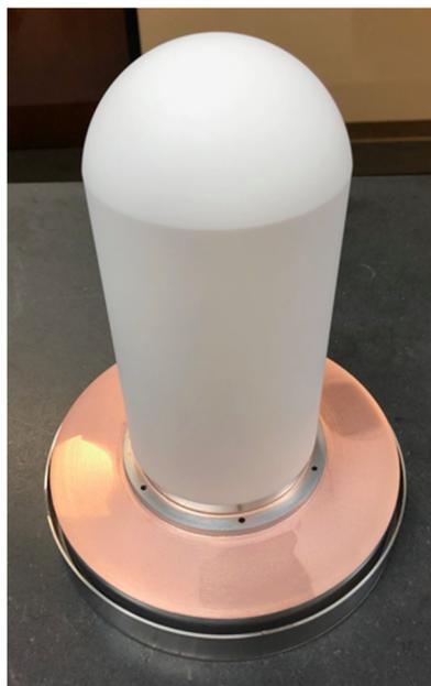
Figure 3: Output window braze completed awaiting TiN coating.
