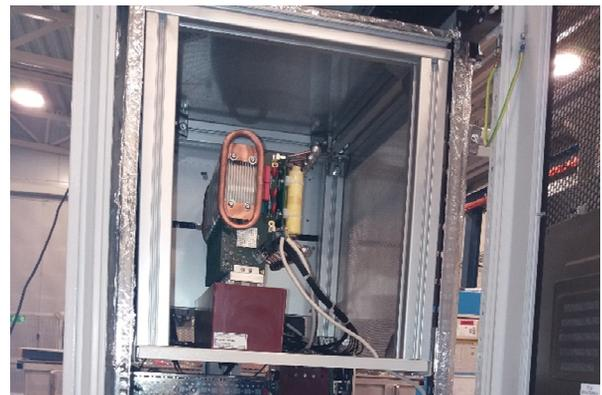
Figure 3: HV Switch in the ESS modulator prototype.
