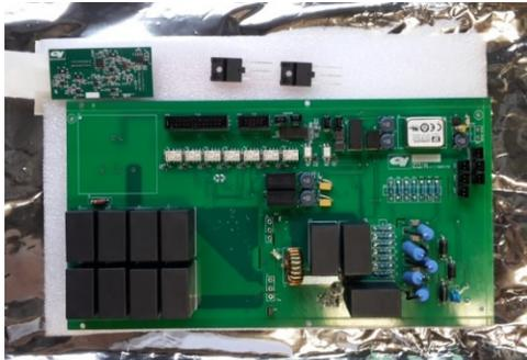
Figure 4: G2 PSU and control prototype boards.
