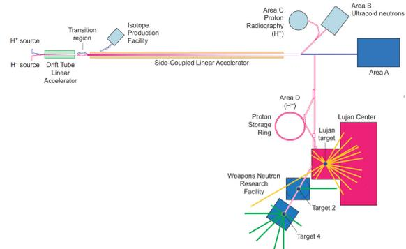
Figure 1: Pictorial Representation of LANSCE.
