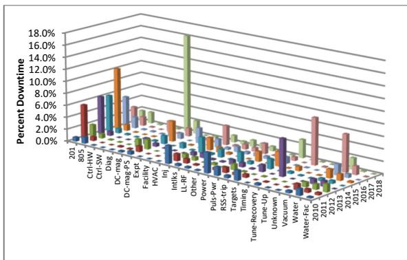
Figure 3: Annual Downtime Data for Target 1, Binned by SSC: DTL = 201, CCL = 805.
