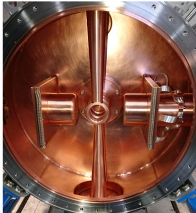
Figure 3: Rebuncher inside view.
