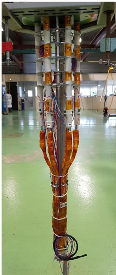
Figure 6: Current leads on SPTS top plate.
