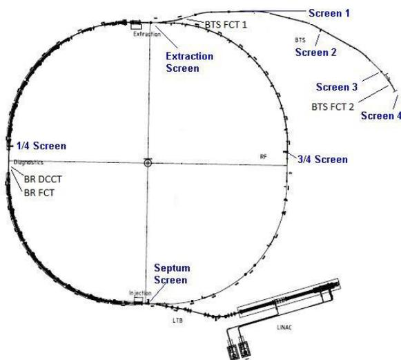
Figure 1: Booster and BTS instrumentation.
