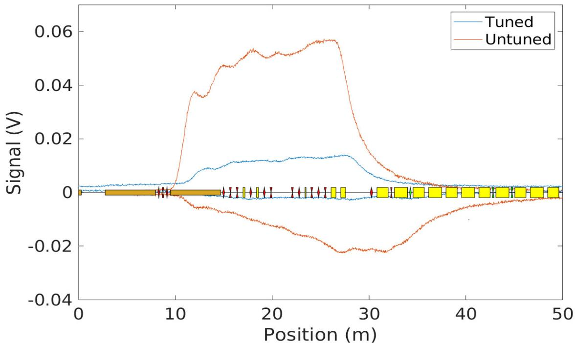
Figure 3: Linac and LTB OBLM signal. Top two traces are losses on the outside fibre, bottom two are losses on the inside fibre.
