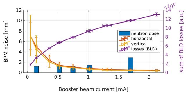
Figure 2: BPM reading error vs injected current.
