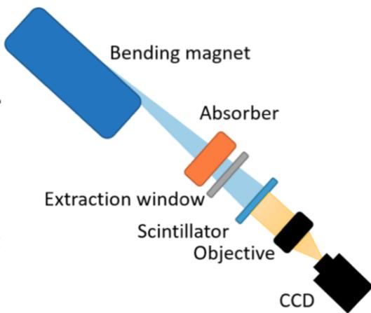
Figure 6: Experimental setup: the synchrotron radiation produced by a dipole is filtered by a copper absorber and extracted through an extraction window. The radiation is converted into visible light by a scintillator and imaged onto a CCD camera by an objective.
