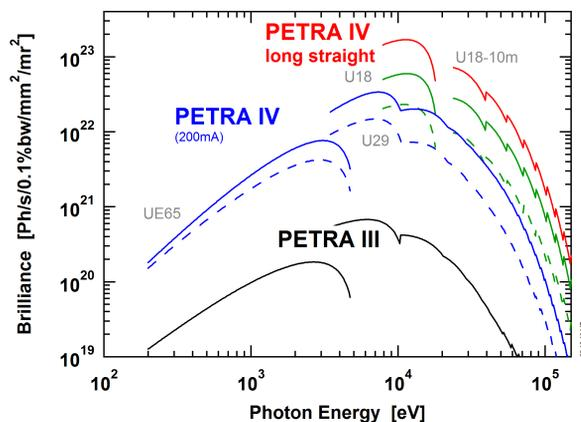
Figure 2: Spectral brightness for a current of 200 mA (blue, green, and red curves) in comparison with PETRA III (black curves) for a ring current of 100 mA. Comparison for a 5mUE65 undulator (P04 beamline at PETRA III) for soft x-rays, and a 5 m U29 undulator (P10 beamline at PETRA III) for hard x-rays. The solid lines correspond to the high-brightness/high-coherence mode, and the dashed lines to the timing mode. Additionally, gains from a 5 m and 10 m long U18 undulators are shown.
