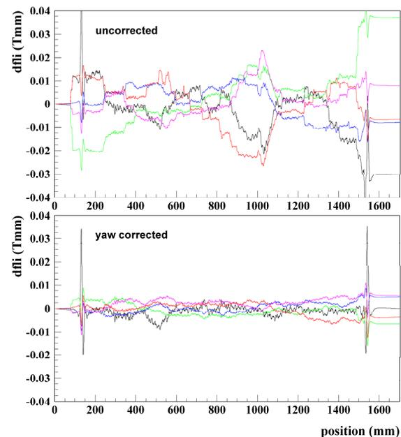
Figure 2: Individual differences to an average of five period-filtered 1<sup>st</sup>-field integrals without (top) and with yaw-correction.
