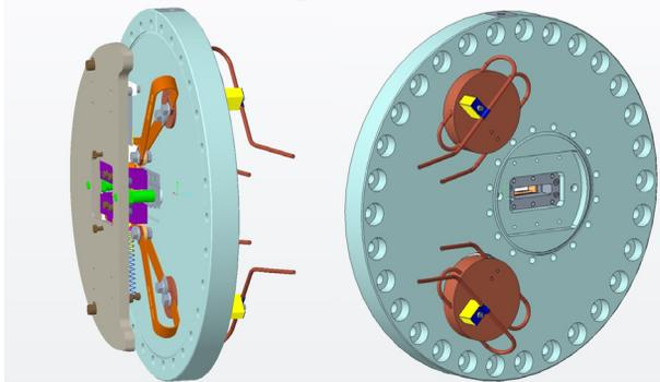
Figure 6: Water cooling of the flexible taper sections.
