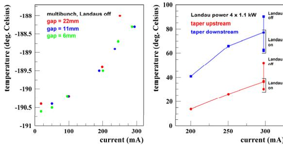
Figure 5: Left: Temperature of the magnet girder versus current for several gaps. Right: Temperatures of the flexible tapers versus current. “Landau on” includes also optimization of main cavities. Landau power means the power, which is deposited into the cooling water.
