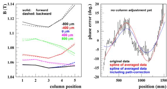
Figure 3: Left: Fitted effective fields at several vertical and longitudinal positions and for different scan directions. The longitudinal positions coincide with the locations of the columns, which support the in-vacuum girders. Right: phase errors from original and from simplified splined data (for details see text).
