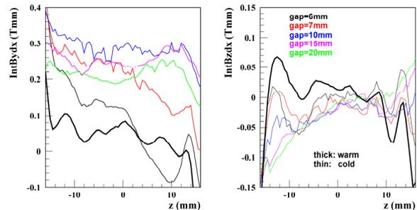
Figure 1: Vertical (left) and horizontal field integrals of CPMU17.
