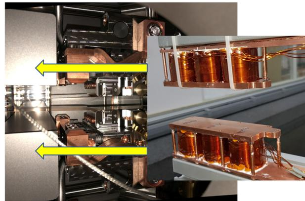
Figure 4: Two inserts (arrows) in the taper section housing the water-cooled air coil arrangement.
