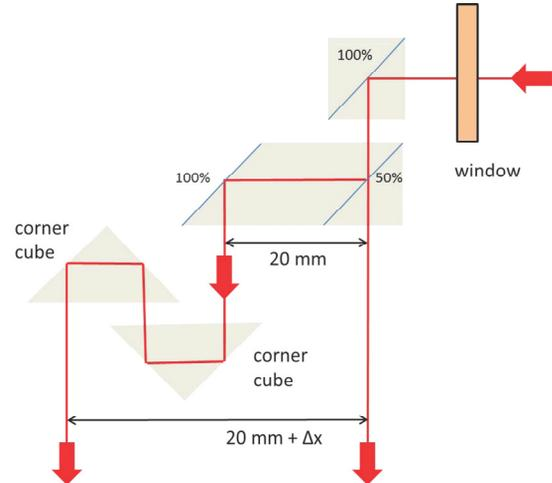
Figure 7: Generation of two parallel laser beams for HZB-SAFALI. The additional separation is:  $\Delta x = 45\text{mm}$ .
