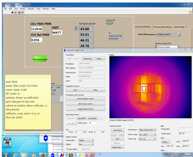
Figure 3: Measurement screenshot of the high-power RF test of the VSR HOM load prototype ID02.
