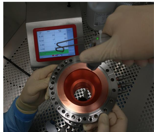
Figure 5: Prototype of the CsB during particulate counting in the clean room, revealing modest emission rates.
