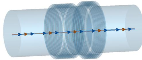
Figure 8: Simulation model of the MeB, featuring two separate segments of slightly different diameters. The straight part in between will be tuneable by an active linear mover and also be used as cooling intercept.
