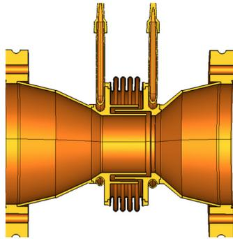
Figure 7: CsB modified with additional welded and copper-coated tapers (PrepCsB) to be mounted in between the two 1.5 GHz cavities used in the preparation phase test module (cf. Fig. 1).
