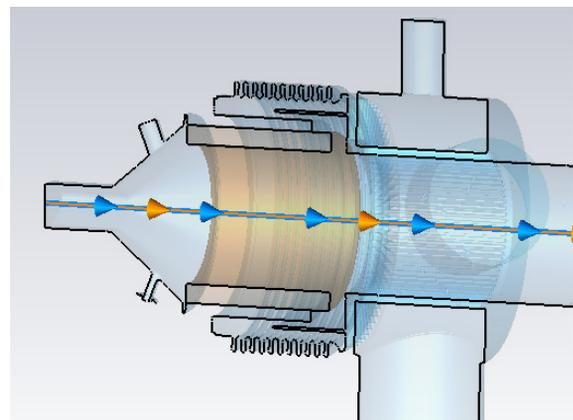
Figure 2: Cross section of the modified Warm End Group
