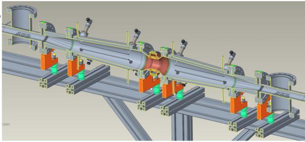
Figure 6: Setup of the CsB beam experiment to be installed at BESSY II during the upcoming shutdown. The CsB will be accompanied by tapers equipped with stripline-like couplers needed to monitor and damp wake power deposited in the area.
