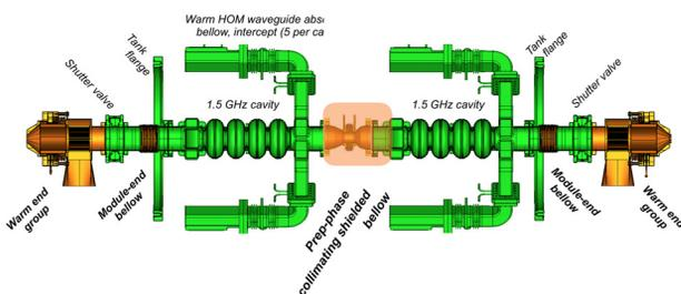
Figure 1: Prep(ARATION) phase VSR cold string set up, featuring only two 1.5 GHz cavities and a modified central bellow, otherwise being identical to the final module set up (cf [1], Fig. 1).
