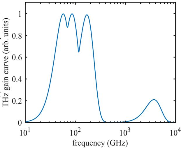
Figure 2: Calculated accessible frequency range of laser-induced THz radiation over four revolutions given by the gain curve  $g^2(f)$  (see Eq. 2).
