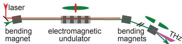
Figure 1: Setup for the coherent emission of laser-induced THz radiation (see text for details).
