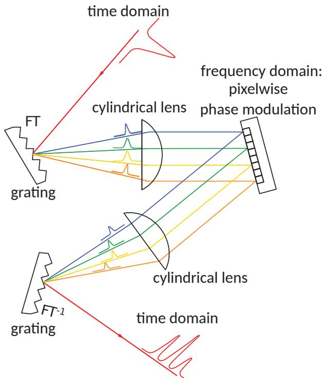
Figure 4: Temporal shaping of a laser pulse is possible by optically mapping the beam onto the Fourier plane and introducing a frequency-selective phase shift. The angles and distances are not to scale.
