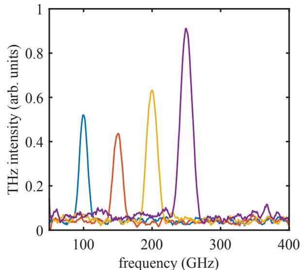
Figure 5: Narrowband sub-THz spectra acquired using a spatial light modulator.
