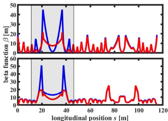
Figure 3: Horizontal (top) and vertical (bottom) beta function  $\beta$  versus longitudinal position  $s$  of the present optics (blue) and the future EEHG optics (red). Inside the modified area (gray), the maximum beta function is reduced by more than a factor of two. Elsewhere, the beta function does not change significantly.
