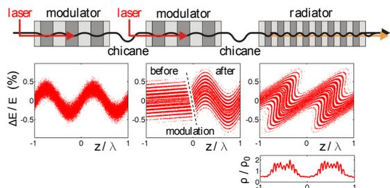
Figure 1: Magnetic setup for EEHG, the corresponding longitudinal phase space distributions and the final longitudinal electron density.
