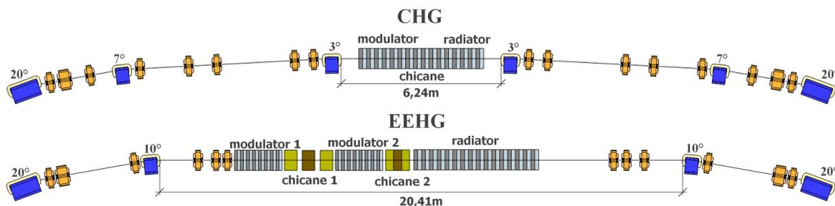
Figure 2: Present (top) northern part of the storage ring with an undulator separated into three parts used for CHG and the future modifications to enable a long straight section for EEHG (bottom) with dipoles in blue and quadrupoles in orange.
