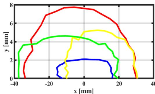
Figure 5: Dynamic aperture for on-momentum particles (red), 1% and -1% momentum offset (yellow, green) for the future optics compared to the present on-momentum dynamic aperture (blue). The off-momentum apertures are centered at the dispersion orbit.
