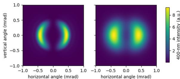
Figure 6: Angular distribution of undulator emission at 400 nm of an undulator tuned to 775 nm (left) as simulated with *SPECTRA* [9]. Convoluting the distribution with a 2D Gaussian representing the laser beam divergence results in a realistic distribution of a laser-induced signal (right).
