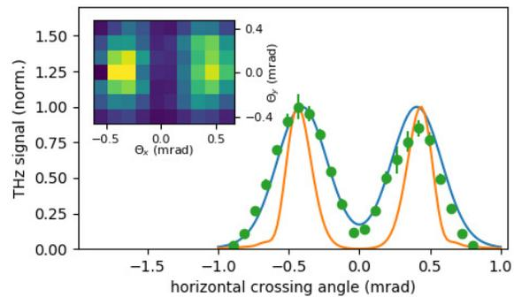
Figure 7: Normalized THz signal (dots) under variation of the horizontal crossing angle at a vertical crossing angle of  $0^\circ$  together with *SPECTRA* simulations without (orange) and including (blue) the laser divergence (see Fig. 6). Inset: THz signal under coarse variation of the horizontal and vertical crossing angles  $\theta_{x,y}$  (top left).
