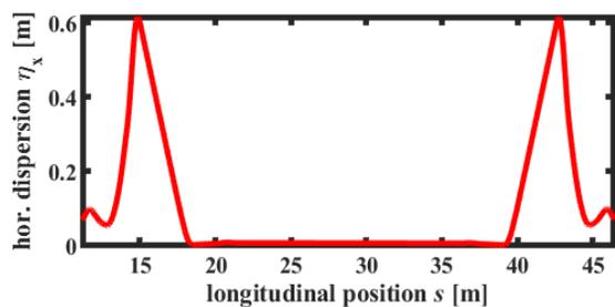
Figure 4: Horizontal dispersion  $\eta_x$  versus longitudinal position  $s$  in the EEHG section. The residual dispersion is smaller than 1 mm in the straight section.
