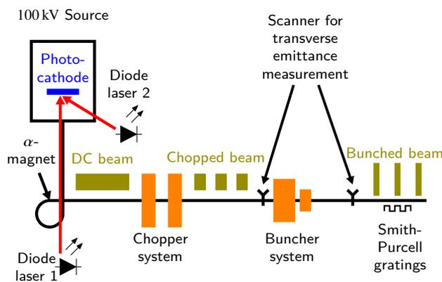
Figure 1: Scheme of the test setup.
