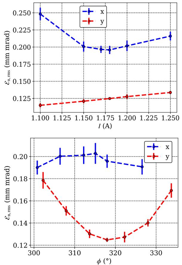
Figure 3: Emittance growth due to wrong magnetic field of the double solenoid (top) and wrong rf phase of the second chopper cavity.
