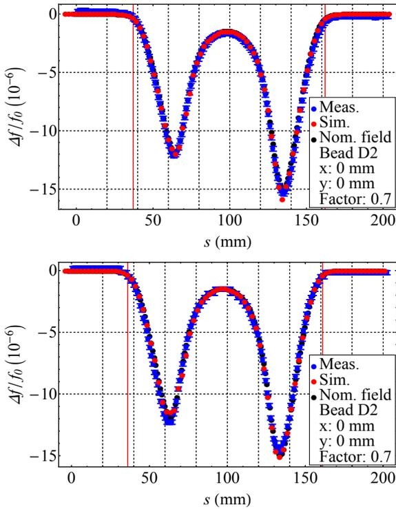
Figure 2: Measurements and simulations of the electric field on the reference axis in the chopper cavities.
