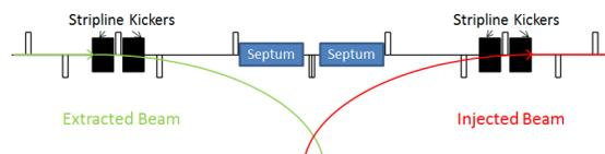
Figure 2: Schematic of the PETRA IV injection and extraction section.
