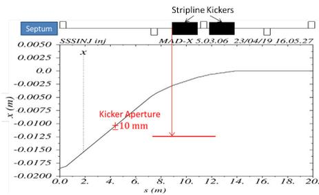
Figure 3: The horizontal trajectory of the injected beam.
