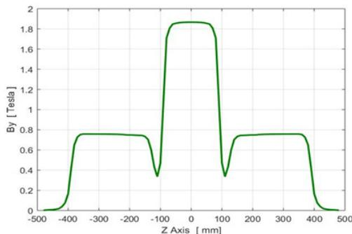
Figure 3: LG dipole magnet profile.
