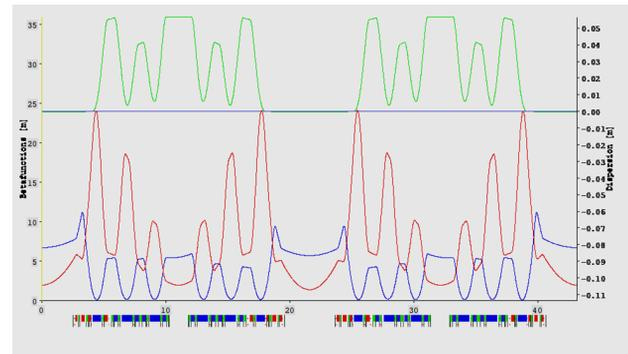
Figure 4: The S6BA\_E lattice with LG dipoles (2-4 from left at each achromat) and reverse bend quadrupole / dipoles.
