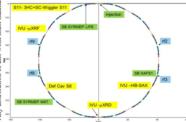
Figure 5: Machine geometry indicating the positions of the super-bends, some IDs and the rf cavities.
