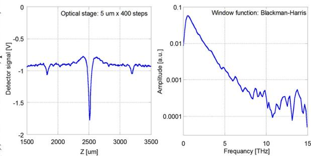
Figure 1: (Left) Measured interferogram of transition radiation and (Right) Radiation spectrum.
