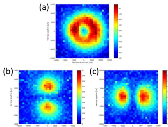
Figure 2: (a) Measured spatial distribution of CTR without the wire grid polarizer. (b) and (c) are measured vertical and horizontal components of CTR.
