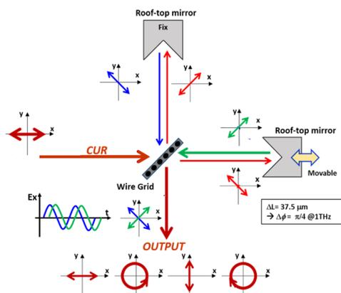
Figure 4: Polarization controller employing a Martin-Puplett interferometer.
