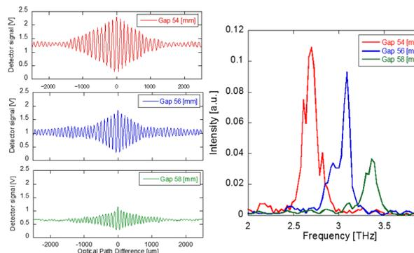
Figure 3: (Left) Interferogram and (Right) spectrum of coherent undulator radiation with different gaps.
