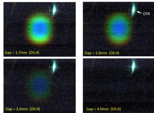
Figure 5: Observed the undulator radiation with different gap using a color CCD camera.
