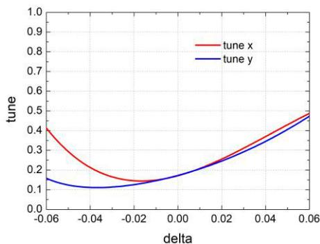
Figure 9: Tune shifts with momentum (28-cells case).
