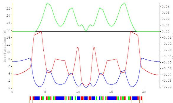
Figure 2: IDB-7BA lattice of the design with 30 cells.
