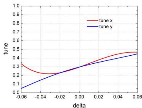
Figure 5: Tune shifts with momentum (30-cells case).
