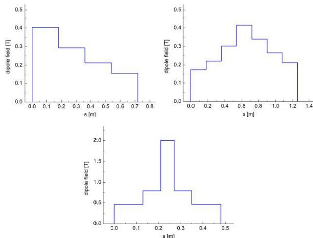
Figure 3: Longitudinal gradient dipole field profiles of the first (upper left), the second (upper right) and the middle (lower) bends. The last two LGBs in the lattice have the same field profiles as the first two ones but with reverse variation.
