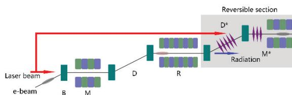
Figure 1: Layout of the reversible SSMB.
