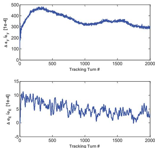
Figure 4: The growth of vertical emittance and energy spread.
