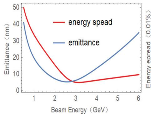
Figure 9: The emittance and energy spread evolution.
