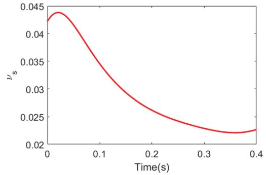
Figure 5: synchrotron tune curve in ramping process.
