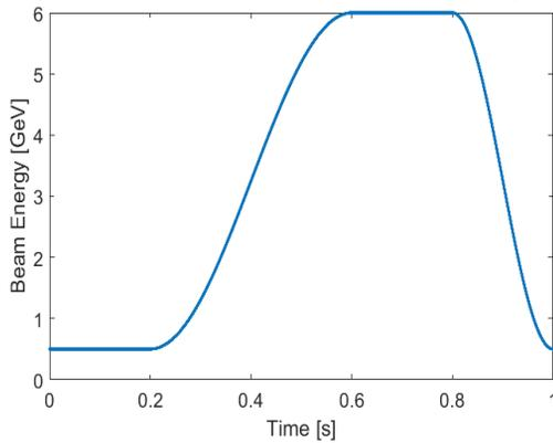
Figure 3: An energy ramp cycle of HEPS booster.
