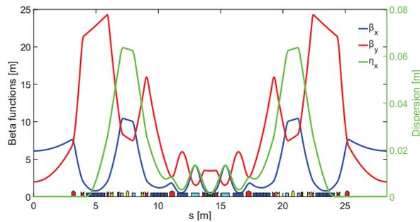
Figure 2: Linear optical functions and magnet layout of the selected lattice. In the magnet layout, bends are in blue and cyan (RBs), quadrupoles in red, sextupoles in yellow and octupoles in brown.
