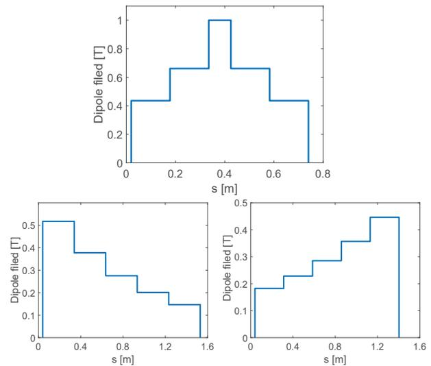
Figure 3: Dipole field profiles of the third (upper), first (left lower) and second (right lower) LGBs. The profiles of the fourth and fifth LGBs are mirror-symmetrical with the second and first ones.
