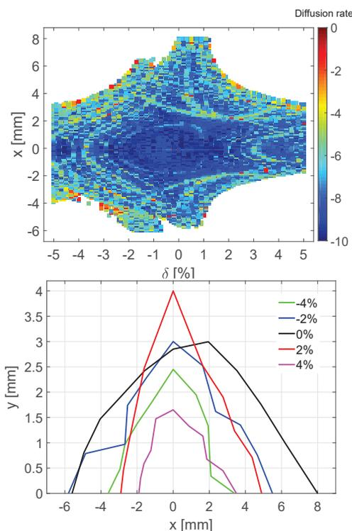
Figure 6: Horizontal DAs for different momentum deviations (upper) and off-momentum DAs (lower).
