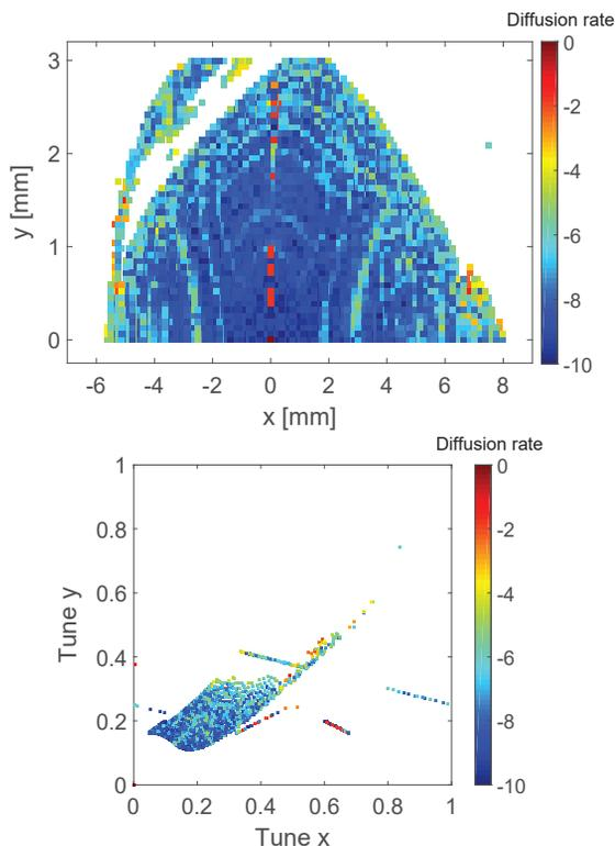
Figure 4: FMA of the optimized DA, tracked at the middle of long straight sections with  $\beta_x$  of 6.11 m and  $\beta_y$  of 1.98 m. Upper: x-y space. Lower: tune space.
