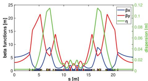
Figure 4: Linear optical functions and magnet layout of the designed hybrid 7BA lattice.
