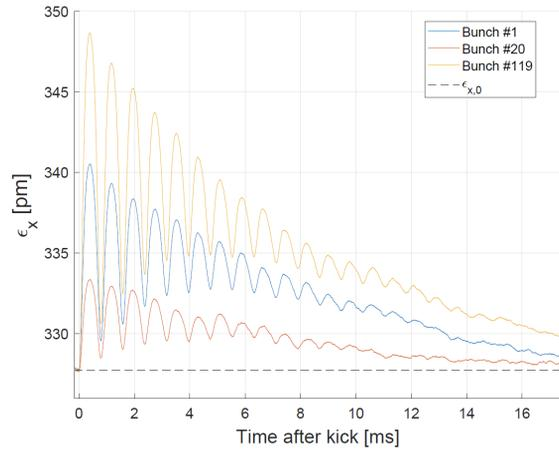
Figure 3: Emittance growth of bunches #1, #20 and #119. After the initial kick, the emittance increases to a maximum, followed by modulation with the synchrotron frequency by de-/recoherence due to the finite chromaticity.
