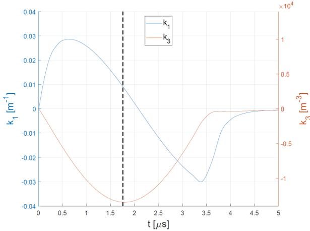
Figure 2: Temporal evolution of normalized, integrated quadrupole and octupole components. The black dotted line indicates the time at which the injected bunch arrives at the MIK. Dynamic stored beam perturbations are due to the non-zero quadrupole components.
