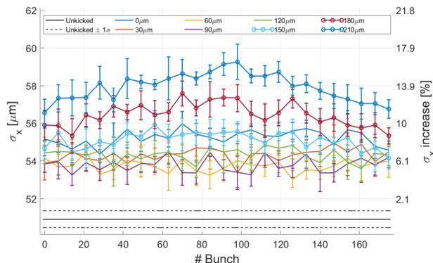
Figure 5: Bunch-by-bunch width measurements for different closed-orbit bump amplitudes through the MIK. The minimum increase is found at bump sizes between 60-90  $\mu\text{m}$ . The user operation orbit has now been adjusted to have a 100  $\mu\text{m}$  bump leading to a beam size increase of  $\approx 6\%$ , which is within stable operation of MAX IV 3 GeV. Significant differences in the beam size increase on bunch-by-bunch basis are only seen for large bumps.
