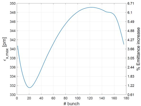
Figure 4: Maximum bunch-by-bunch emittance. The growth of the emittance varies significantly between bunches, with a maximum growth at bunch #120 of  $\approx 6.5\%$ . The difference stems from the difference in quadrupole field seen by each bunch
