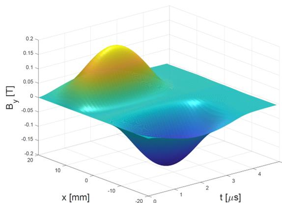
Figure 1: Temporal shape of the magnetic field from the MAX IV Multipole Injection Kicker with a  $5 \mu\text{m}$  Ti-coating. Peak field is reached after and  $1.76 \mu\text{s}$ .
