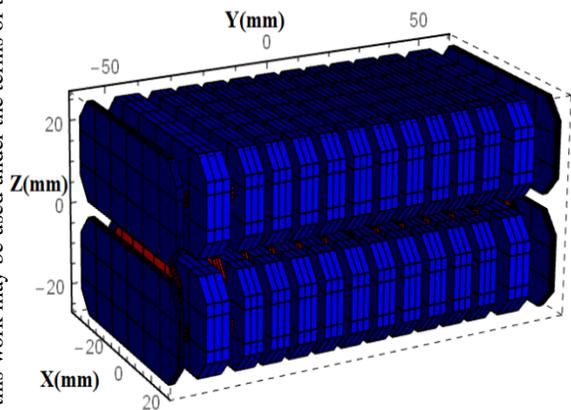
Figure 2: Magnetic model of U17 undulator, modelled by Radia [4].
