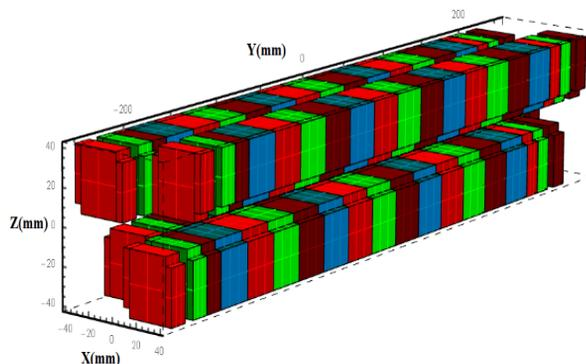
Figure 3: Magnetic model of U114 undulator, modelled by Radia [4].
