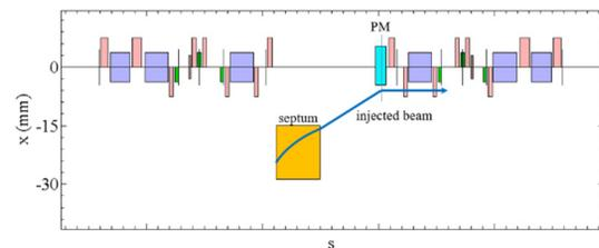
Figure 6: SPS-II storage ring injection based on a PM.
