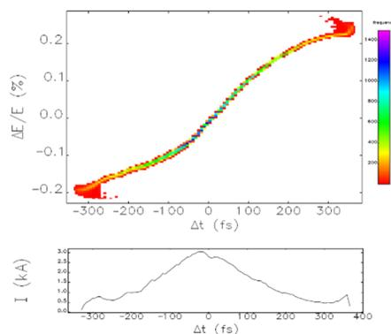
Figure 5: Longitudinal phase space (top) and distribution (bottom) after L2.
