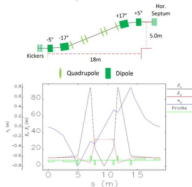
Figure 4: Layout of the TL (top) and optics function along the TL (bottom).
