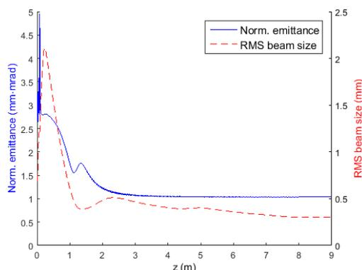
Figure 3: Normalised transverse emittance (blue, solid line) and beam size (red, dashed line) from the ASTRA simulation of the low energy beam section.
