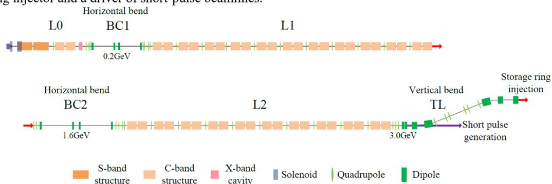
Figure 1: Layout of a full energy injector linac for SPS-II including a vertical transfer line to the SPS-II storage ring.
