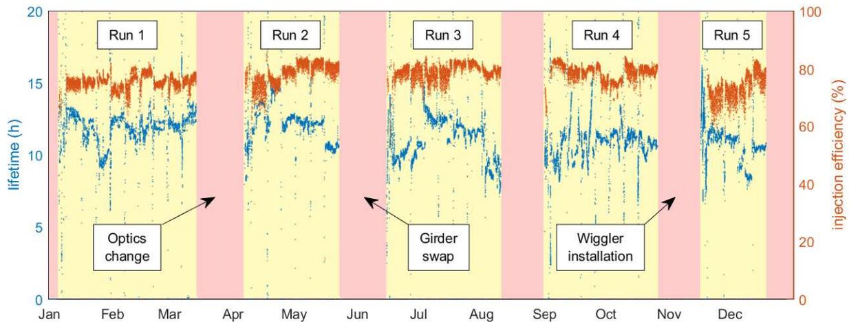
Figure 4: Lifetime and injection efficiency during 2018. Sustained drops in lifetime coincide with hybrid filling patterns (when bunch charge is higher and are therefore independent from the DIAD modifications), and periods of large variability occur during machine development days.
