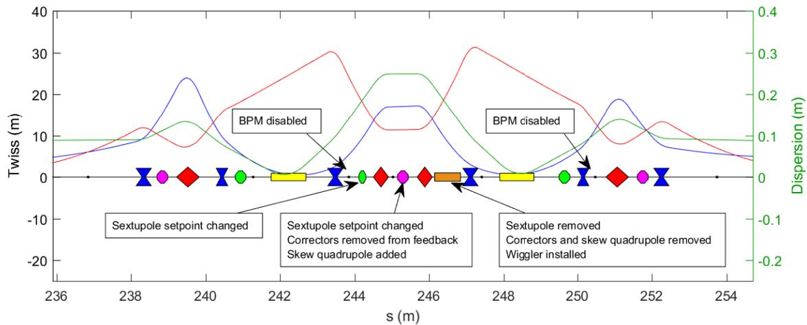
Figure 3: Summary of changes required in the local DBA cell to accommodate the DIAD wiggler.
