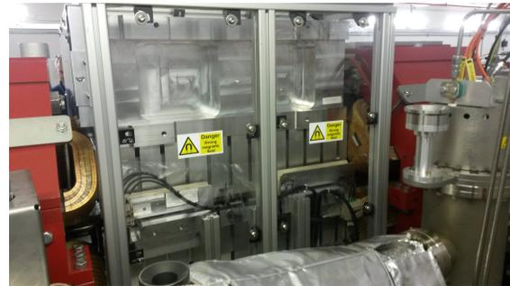
Figure 1: DIAD wiggler installed between two quadrupole magnets in the centre of a DBA cell.
