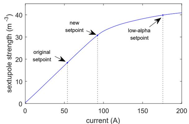
Figure 2: Strength as a function of current for the remaining defocussing sextupole magnet.
