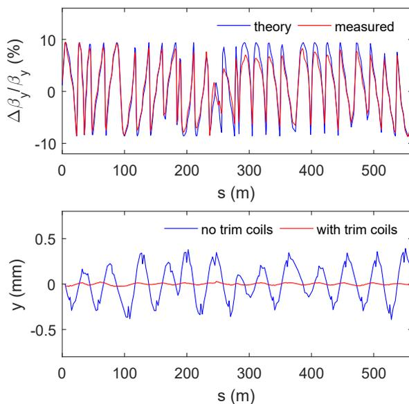
Figure 5: Vertical beta-beat (top) and orbit distortion (bottom) introduced by the DIAD wiggler.
