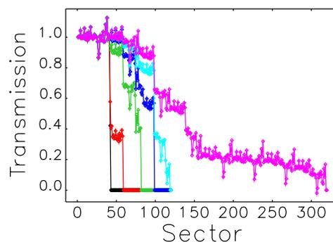
Figure 2: Beam transmission improvement by equalizing the coordinates at the end of sector 40 to the coordinates of the injected beam. Several iterations are shown, one turn equals 40 sectors.
