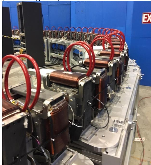
Figure 4: Details of one the FFA arc magnets.
